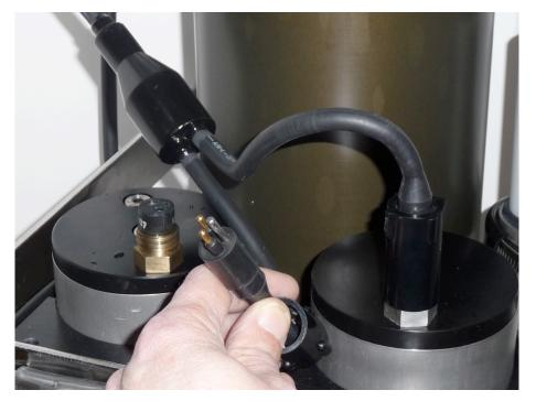
This connector is "live" with the voltage from the first battery pack. Plug it into the second pack immediately to reduce the risk of short circuits.
